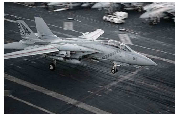
▲ GRUMMAN F-14 TOMCAT LANDING A pilot increases the throttle during touchdown, so that if the aircraft fails to catch the arrestor wires, it still has enough speed to take off again.
